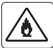
WARNING - Flammable liquid
